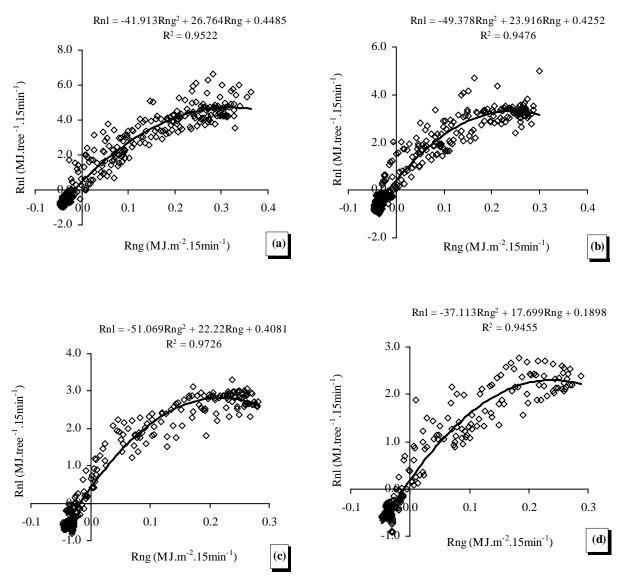
**Figure 4.** Relations between orange canopy net radiation (Rnl) and grass net radiation (Rng) for tree leaf areas of  $37.0 \text{ m}^2$  (a),  $27.3 \text{ m}^2$  (b),  $18.2 \text{ m}^2$ . (c)  $12.0 \text{ m}^2$ , (d), at 15-min time-scale. Period: May-June 2005.
