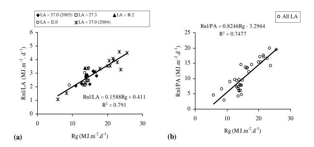
**Figure 6.** Relations between daily values of orange canopy net radiation by leaf area unit (Rnl/LA) and global solar radiation (Rg), with data points being showed separately for each leaf area and the two years (a), and with pooled data between tree net radiation per area unit canopy projected on the soil (Rnl/PA) and global solar radiation (Rg) (b).
